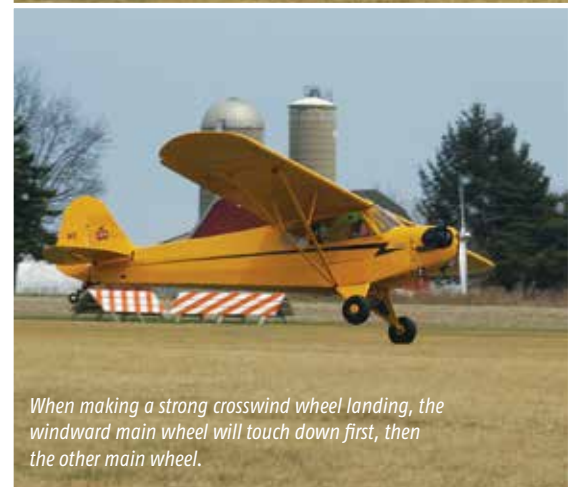
The left wing is held down and right rudder is applied during the flare before touching down.
