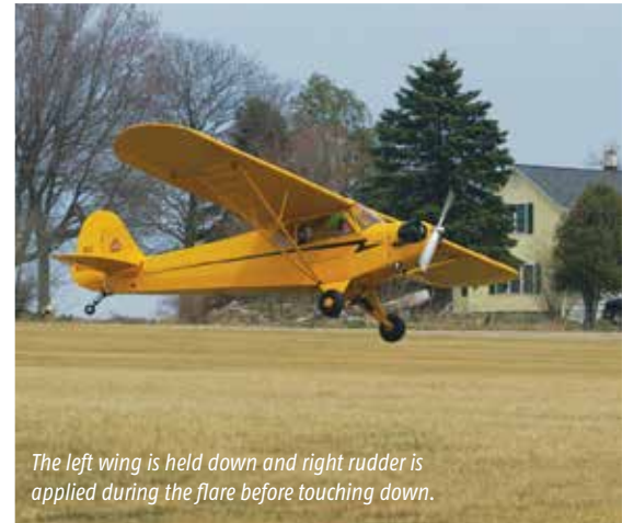
The crosswind is from left to right. Left or windward wing is down and opposite or right rudder is applied to keep the airplane aligned with the runway centerline.
