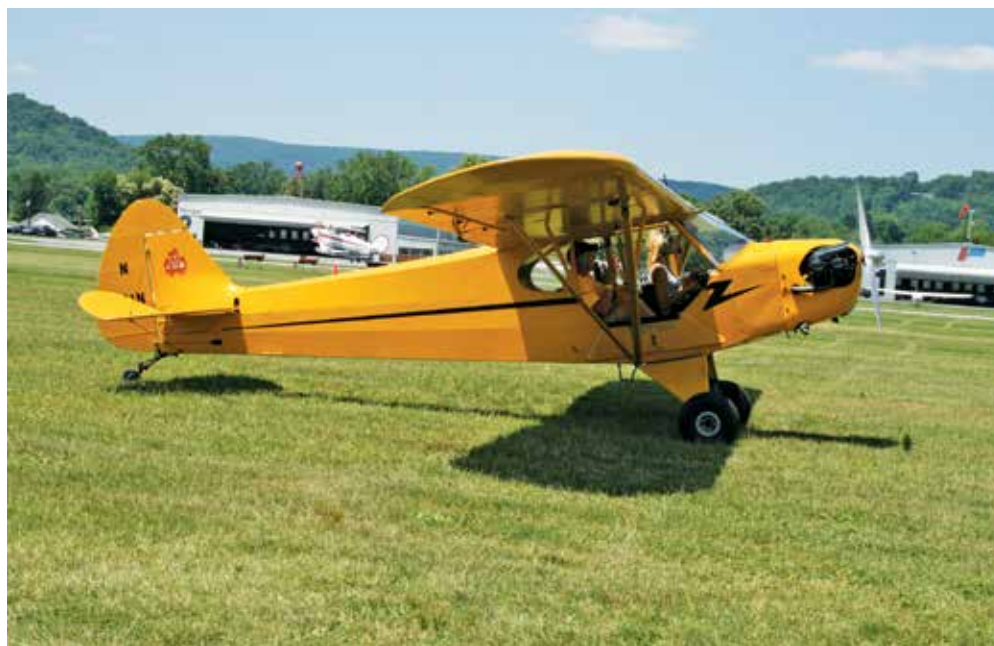
Keep the control stick all the way back with the elevators in the "up" position as smooth power application is made on the takeoff.
