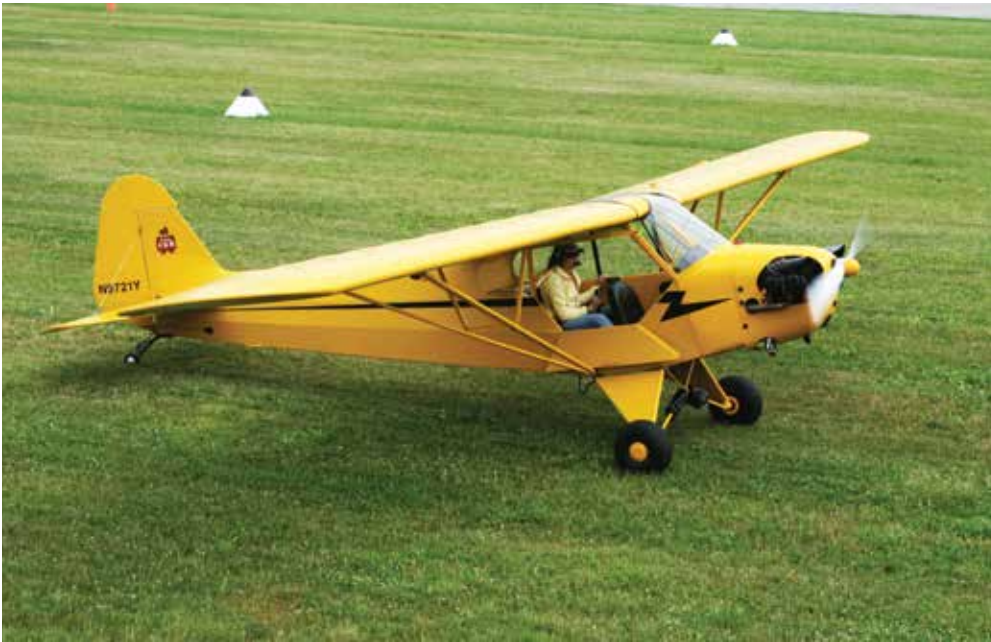
As full power is applied, ease the stick slightly forward. Note the elevators are in the down position helping the tail to become airborne.
