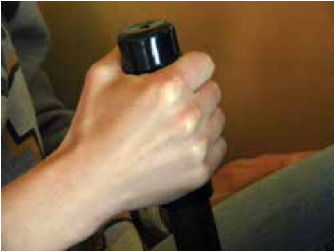
Grasping the control stick too firmly causes poor blood circulation, stiff fingers, and tired, sore forearm muscles. Control inputs will be stiff and mechanical.
