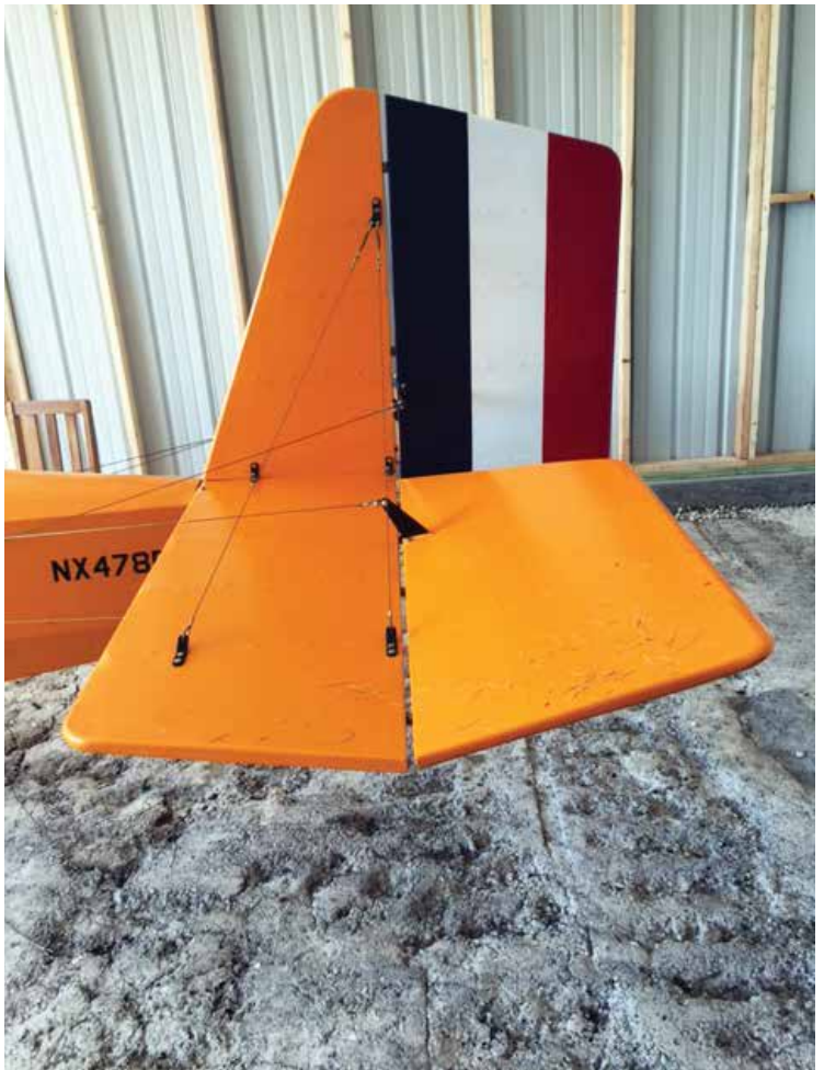
Note the large rudder compared to the vertical fin. A slow-flying aircraft will need more rudder surface to fly comfortably and safely.
