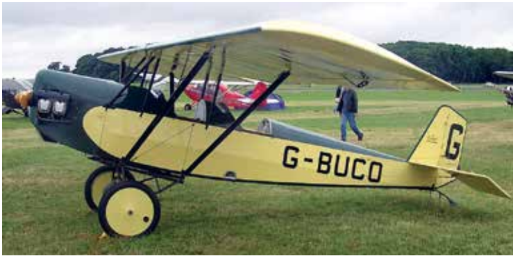
The one-piece wing is straight from wingtip to wingtip and has no dihedral.
