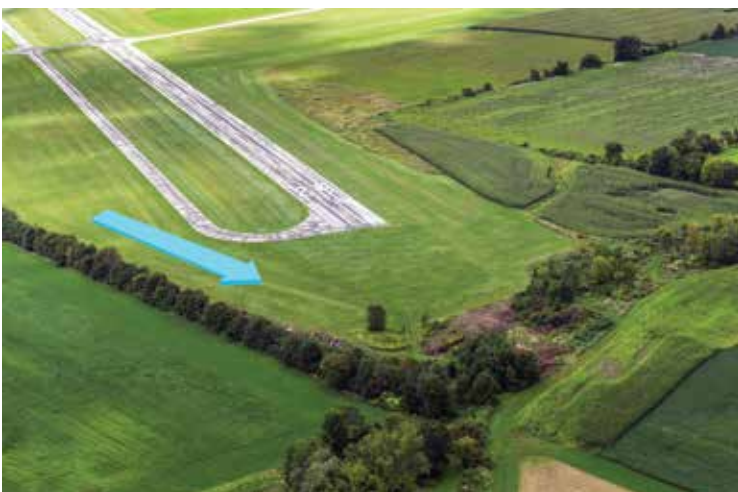
Viewing the approach end of Runway 29, the wind is from about 260 degrees at 12 knots. One can anticipate rolling gusts over the top of the scrub tree line. While on final approach to Runway 29, one can anticipate a dead air area just prior to reaching the tree line followed by some good bumps and updrafts while crossing the tree line.
