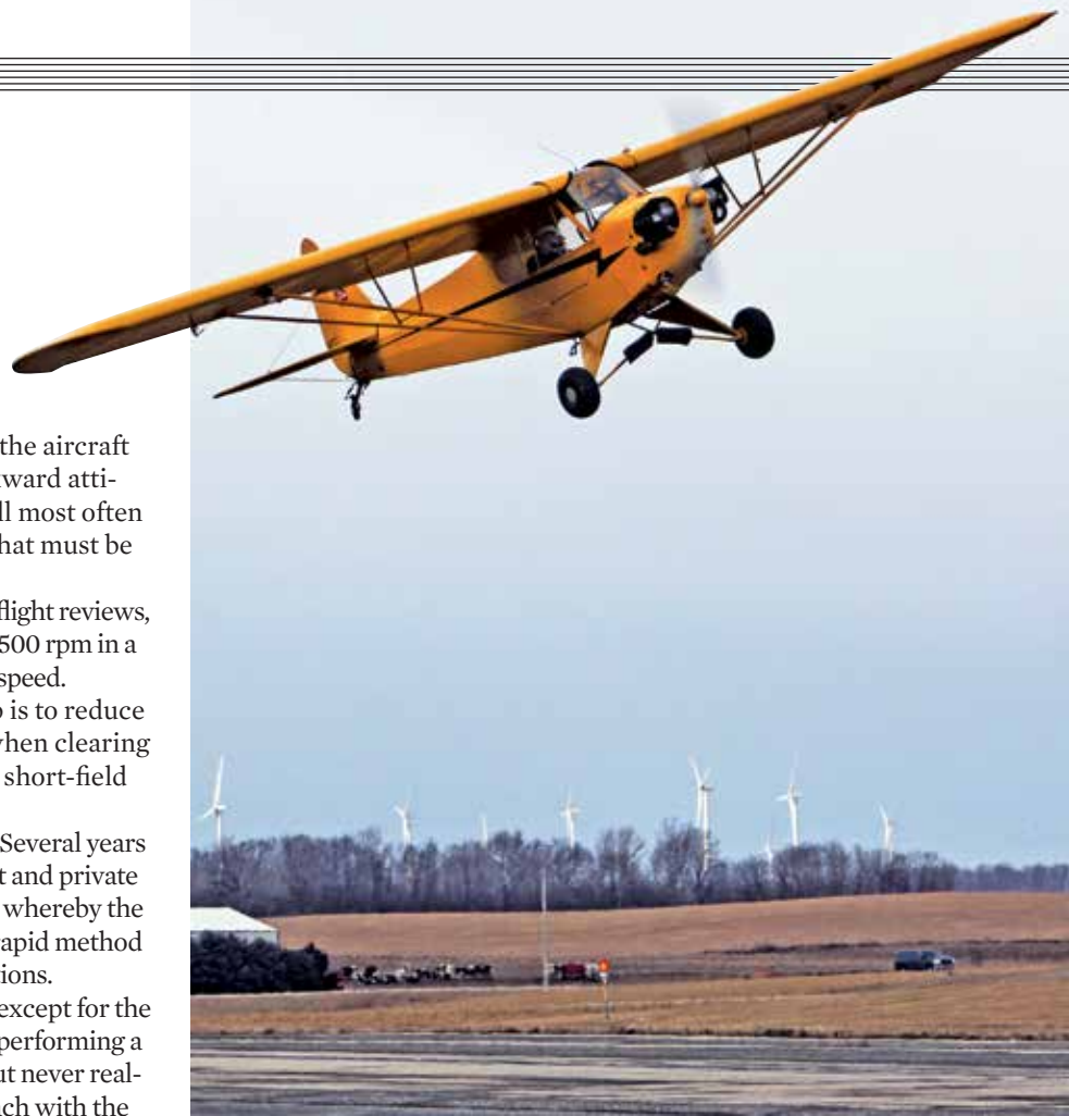
The forward slip used to eliminate excess altitude or clear an obstacle.
