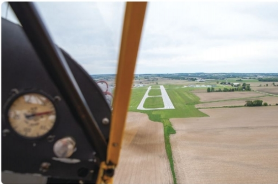
The pilot has turned onto final and is well to the left of the runway centerline. Employing a side slip in this situation allows her to align the aircraft with the centerline in preparation for landing.
