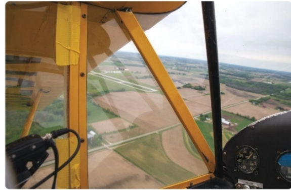
In this situation, the pilot recognizes that he has excess altitude. Rather than waiting until turning final to lose the excess, the inside wing is lowered for the left-hand turn and opposite rudder is applied, causing the aircraft to lose altitude while in the turn. Note how the nose is turned slightly away from the runway.
